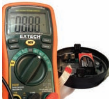
Figure 10. A normal voltage measurement.
