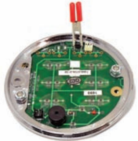
Figure 5. Bypassing a single-battery keypad diode.
