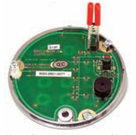
Figure 8. Bypassing a low-profile keypad Schottky diode.
