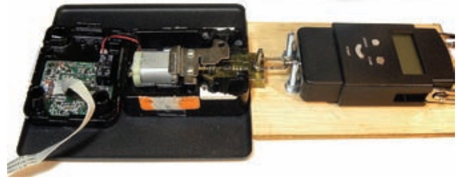
Figure 23. The bolt force testing jig.
